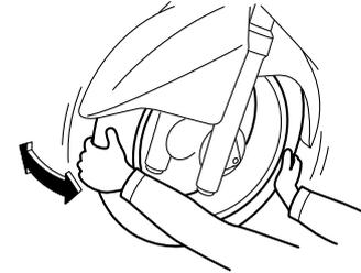
The front and rear wheel bearings must be checked at the intervals specified in the periodic maintenance and lubrication chart. If there is play in the wheel hub or if the wheel does not turn smoothly, have a Yamaha dealer check the wheel bearings.
