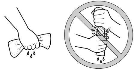
4. Apply oil of the recommended type to the entire surface of the sponge material, and then squeeze the excess oil out.
