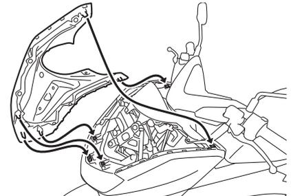
8. Install the windshield by installing the screws.
