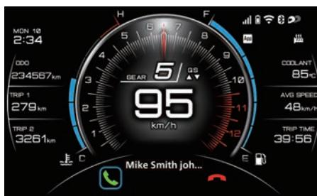
When a phone call is received to a connected smartphone, the ringtone will play through the connected headset and a telephone function will appear at the bottom of the display. Short press enter “
