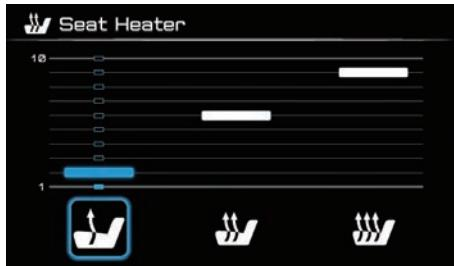
The three seat heater presets can be customized here. Select a preset by operating the joystick left-right and adjust its heat level from 1-10 by operating the joystick up-down. Confirm the settings by short pressing enter “✓” and return to the previous menu.
