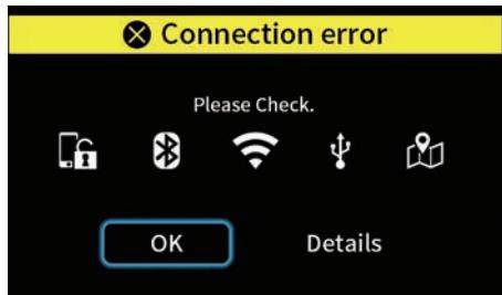
If the navigation system cannot connect to the Garmin Motorize app then this error screen is displayed. Short press enter “
