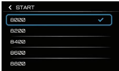
Select the r/min at which the shift indicator light will come on. The operational range is 6000–11800 r/min. It can be adjusted by 200 r/min increments. Confirm the settings by short pressing enter “✓” and return to the previous menu.
