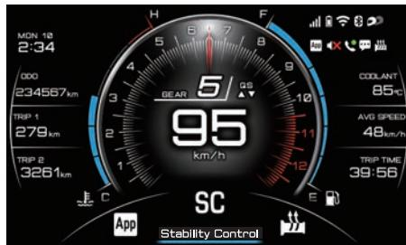
This option turns the stability control systems (“TCS”, “SCS” and “LIF”) on/off together. The stability control system indicator light “**SC**” will come on to indicate “SC OFF” status.
