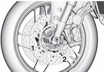
1. Front wheel sensor rotor
