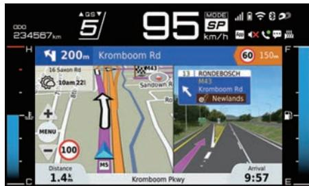
This vehicle is equipped with a navigation system which provides visual and audio (Bluetooth headset required) route guidance. To use the navigation system, you must first download the Garmin Motorize app from an application store onto your smartphone and then register for its paid service.
