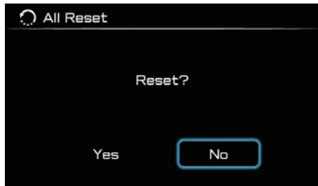
Use this module to reset all machine settings including YRC settings, display brightness, grip warmer presets, traction control, units, and all resettable vehicle information display items.
