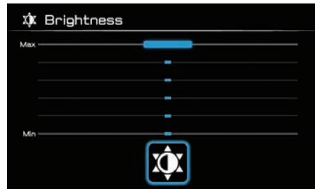
Select the brightness level of the shift indicator light from 1–6 by operating the joystick up-down. Confirm the settings by short pressing enter “✓” and return to the previous menu.
