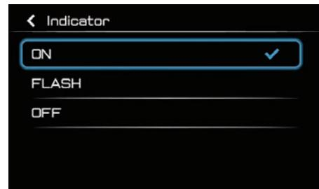
Select “ON” to have the indicator light steadily, “FLASH” to have the shift indicator flash when the indicator start threshold has been reached, or “OFF” to turn the indicator off. Confirm the settings by short pressing enter “
