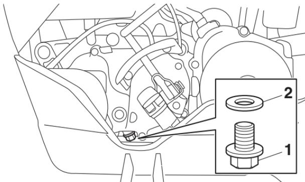
1. Transmission oil drain bolt
