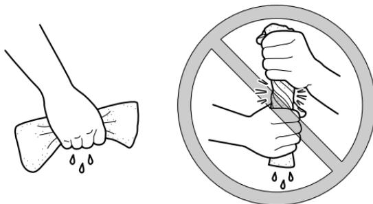
6. Check the air filter element and replace it if damaged.
